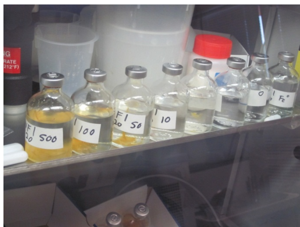
Fig. 9—2000-ppm HPAM-ATBS in 2.85%-TDS water with various \text{FeCl}_3 levels (1-500 ppm), 10-ppb initial \text{O}_2 . Day 0.
