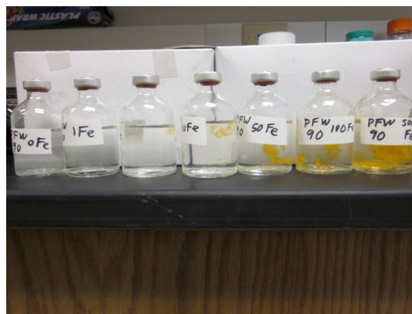
Fig. 10—2000-ppm HPAM-ATBS in 11%-TDS brine with various \text{FeCl}_3 levels (1-500 ppm), 10-ppb initial \text{O}_2 . Day 0.
