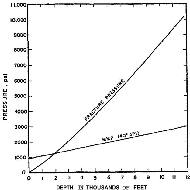
Fig. 7—Increase in CO<sub>2</sub> MMP and fracture pressure with depth for Permian Basin reservoirs. Increasing temperature with depth is incorporated in the MMP correlation shown (from Ref. 33).
