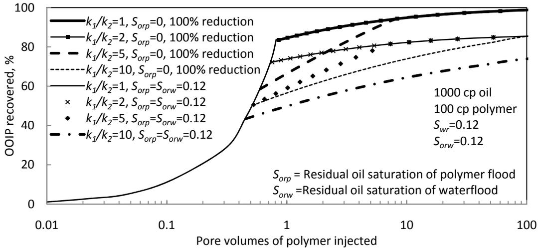
Fig. 9—Effect of heterogeneity. Free crossflow. North Slope case.
