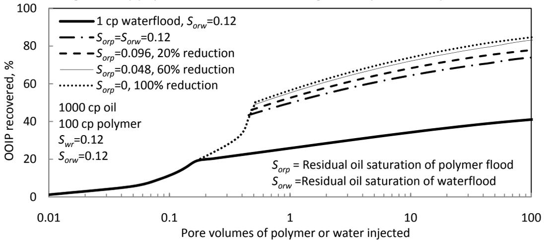
Fig. 6—100-cp polymer flood results for two layers. Free crossflow. North Slope case.
