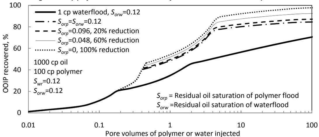
Fig. 7—100-cp polymer flood results for two layers. No crossflow. North Slope case.
