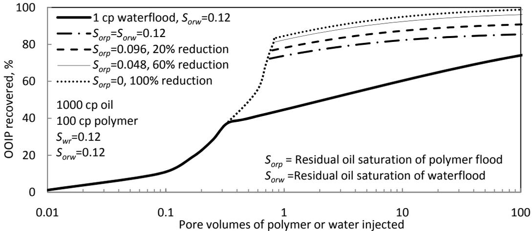
Fig. 5—100-cp polymer flood results for one homogeneous layer. North Slope case.
