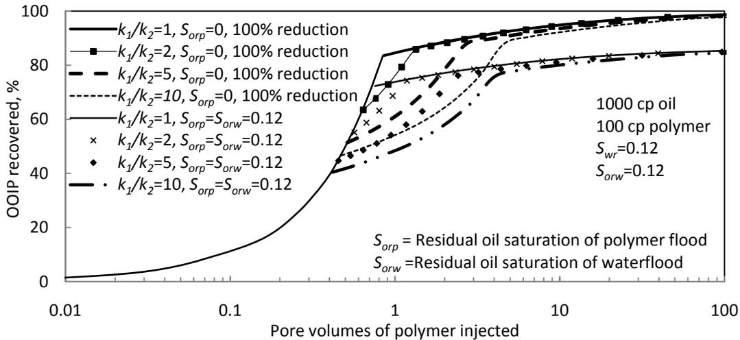
Fig. 10—Effect of heterogeneity. No crossflow. North Slope case.
