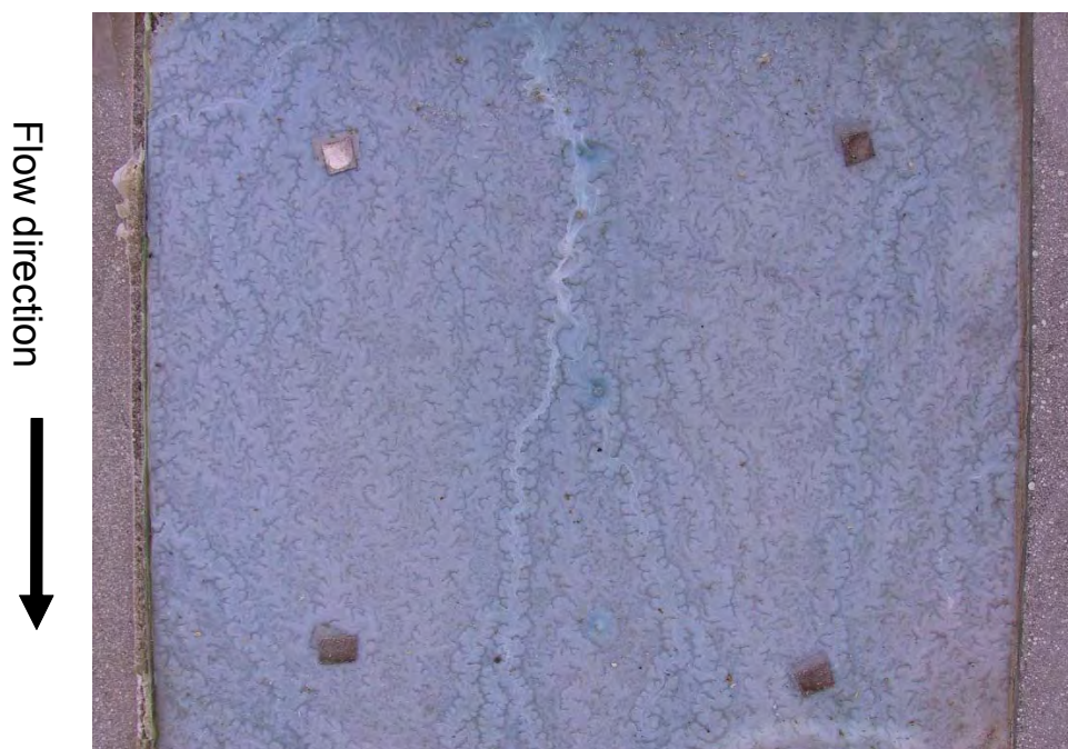
Fig. 15—Wormhole pattern for a guar-borate gel.
